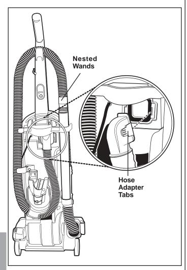
NOTE: Turn off the switch and unplug the electrical cord before clearing hose.
